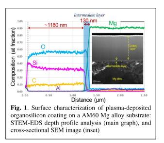
from 5.25 and 6 (P01) to 2.65 and 2.1 (P08), respectively. This difference in the coating chemical composition is primarily due to the higher flow rate of the siloxane precursor that was used in P01 compared to P08 [2]. More importantly, the elemental composition remains relatively constant throughout the entire depth of the coating, as demonstrated in Figure 1.
